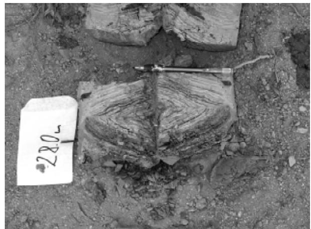
**Photo 3.** Sample from the wavy layered main sliding zone
