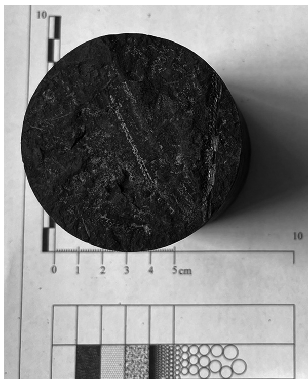
Fig. 3. Core sample photograph with visible graptolites on the bedding surface of a Silurian mudstone.
